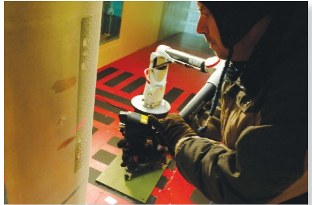
The ROMER Absolute Arm is used to scan the accreted ice on the leading edge of an aircraft wing model.
