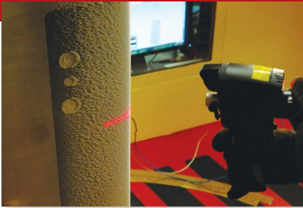
A researcher uses the ROMER Absolute Arm to capture the finer details of the ice shapes.
